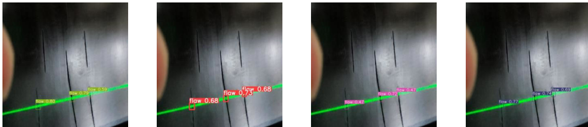
Fig. 9. the detection results from left to right are as follows: YOLOv7-ACMIX, YOLOv5s, YOLOv7-SE, and YOLOv7.
