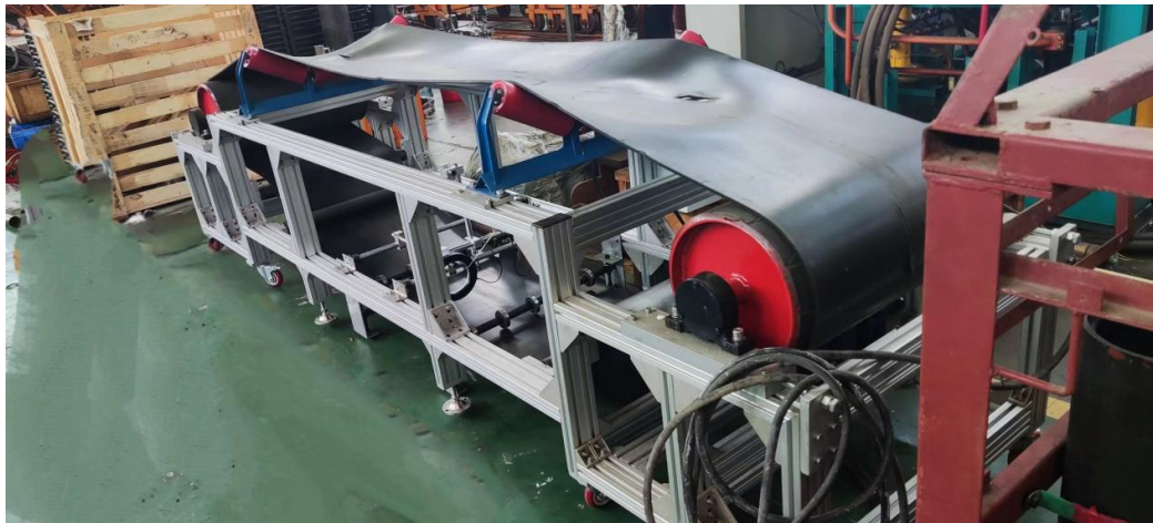
Fig. 1. Conveyor belt test platform physical picture
