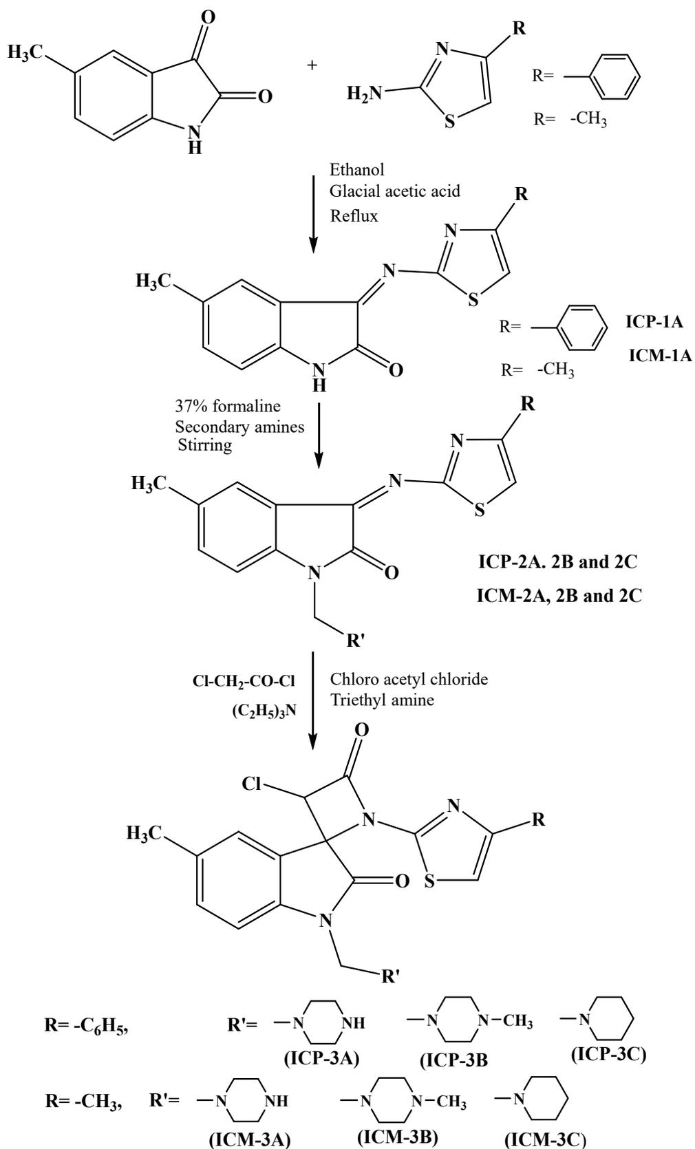
Fig. 1. Reaction scheme of the newly synthesized compounds
