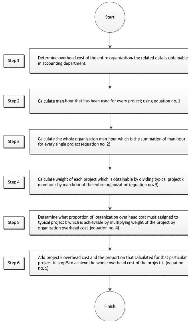
**Fig. 2.** Step by step instruction of company's overhead allocation
