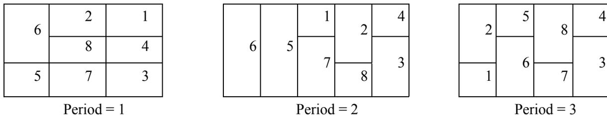
Fig. 3. Flexible bay structure layout configurations for solution encoded scheme shown in Fig. 2
