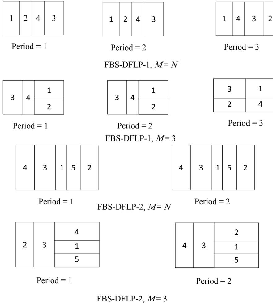
**Fig. 7.** Best layouts found for FBS-DFLP-1 with  $M = N$ , FBS-DFLP-1 with  $M = 3$ , FBS-DFLP-2 with  $M = N$  and FBS-DFLP-2 with  $M = 3$  problems
