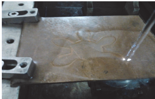
Fig. 1. A gear cut shaped copper plate using Wire EDM
