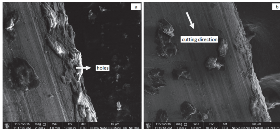
Fig. 2. Micrographs of the brass wire showing (a) holes at 2000X and (b) cutting direction of the wire
