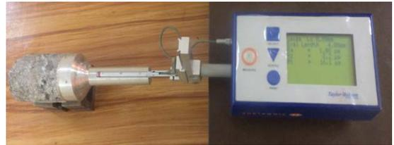
**Fig. 5.** Surface roughness measurement of machined composite bar
