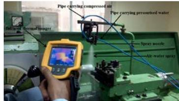
**Fig. 4.** Turning setup in SC machining environment
