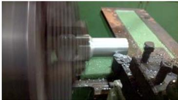
**Fig. 3.** Turning setup in dry machining environment
