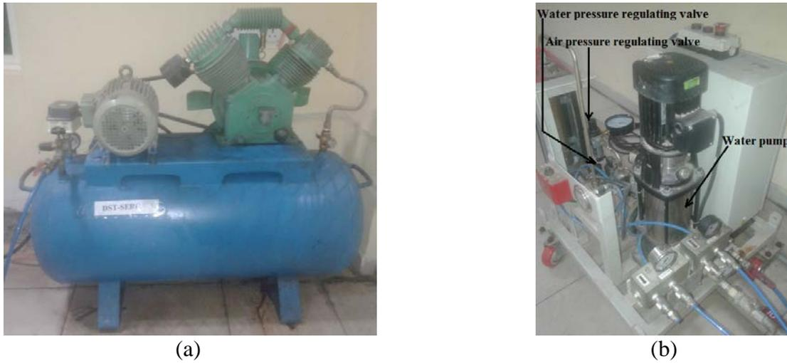
**Fig. 2.** Experimental setup for spray generation consisting (a) air compressor; (b) water pump and pressure regulating valves
