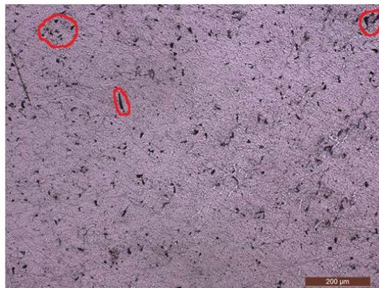
**Fig. 1.** Optical micrograph of AA 7075/SiC composite sample.
