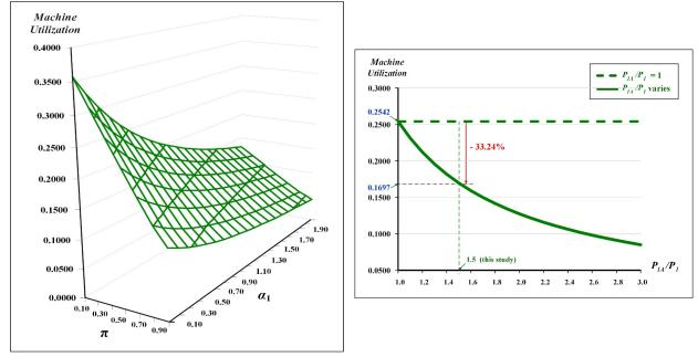
Fig. 15. The collective influences of variations in  $\pi$  and  $\alpha_1$  on Fig. 16. Impact of changes in the ratio of  $(P_{1A} / P_1)$  on machine utilization
