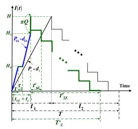
Fig. 1. The inventory status for the proposed buyer-vendor coordination batch system with scrap, breakdowns, overtime, and an external source (in thicker line) compared to a problem with only scrapped items (see the thinner lines)
