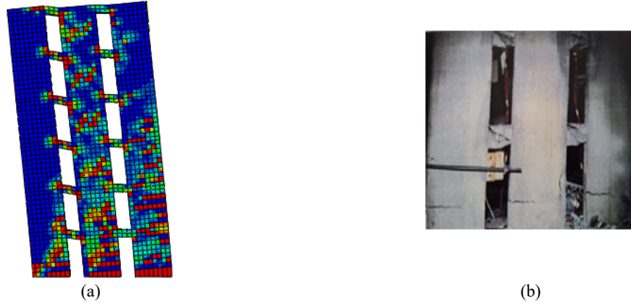
Fig. 7. (a) FEM failure mechanism. (b) experimental failure mechanism (1991)
