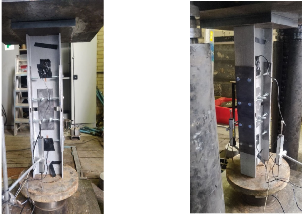
Fig. 4. Manual testing of the models using AMSLER compression testing machine
