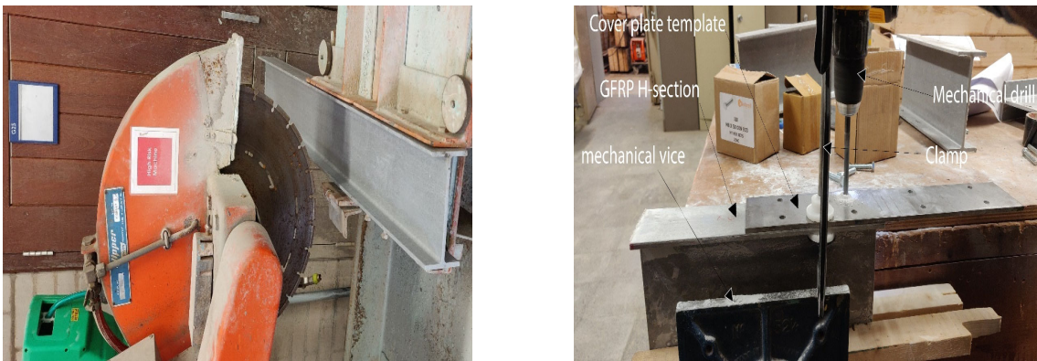
Fig. 3. GFRP H-sections cutting, drilling of holes, and manual model making
