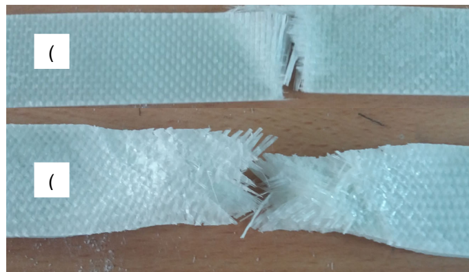
Fig. 12. Failure aspect (a) [0/90] ; (b) [45/-45]
