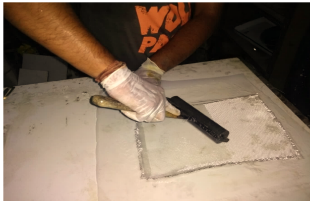
Fig. 1. Fabrication process using hand lay-up method
