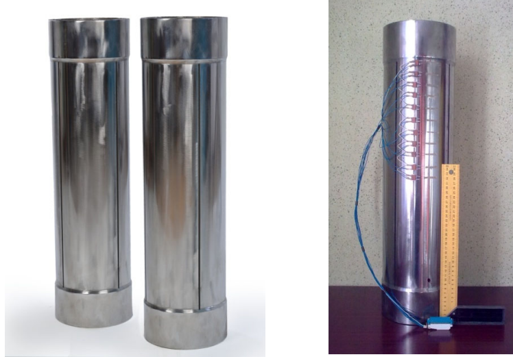
Fig. 10. The bearing link of the resilient element (thin-walled slotted shell with slots)
