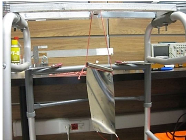
Fig. 7. The free-free boundary condition emulated by suspending the blade by an elastic string
