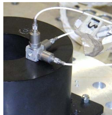
Fig. 4. Three-axis sensors mounted on a battery pack during vibration test
