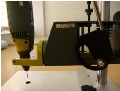
Fig. 11. Precision drill/grinder FBS 240/E Proxxon used in this study
