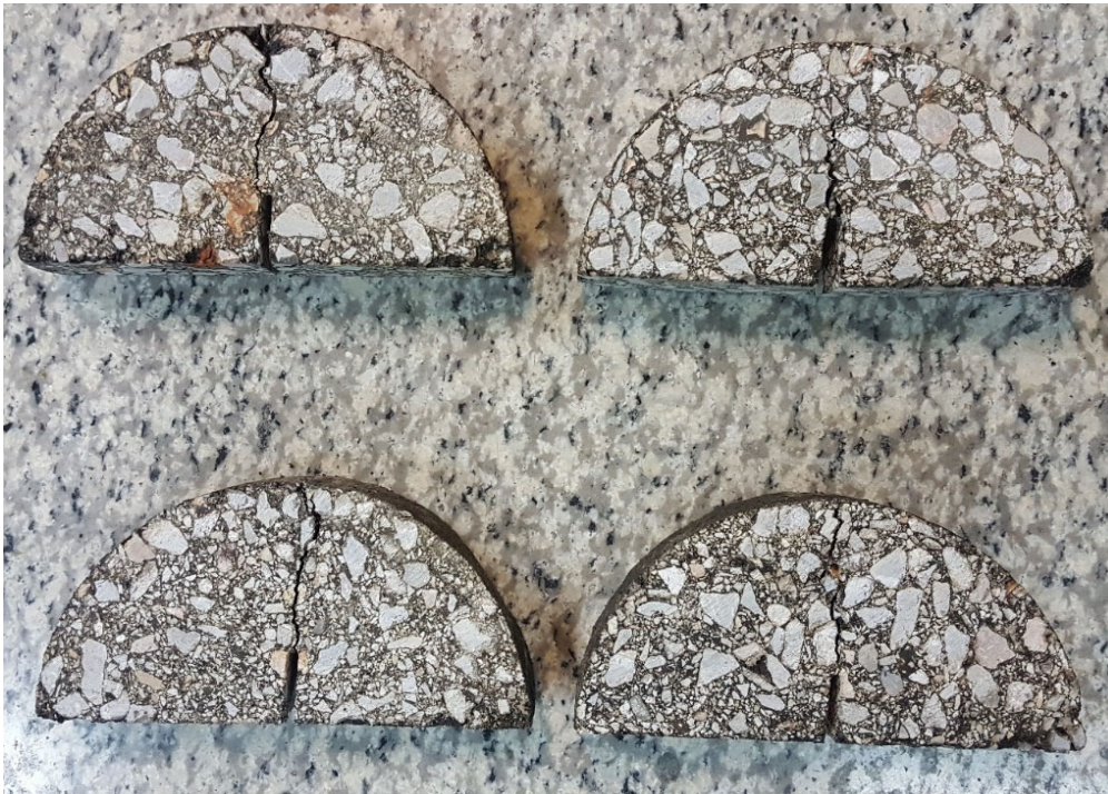
Fig. 10. Propagation path of mode I fracture in the tested asphaltic samples under different testing conditions
