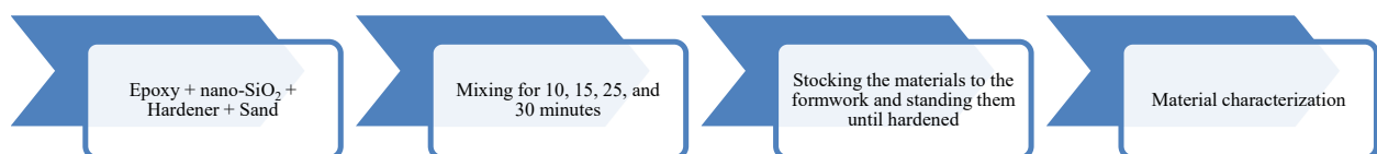
Fig. 1. Flow chart of nanocomposite synthesis with simple mixing method
