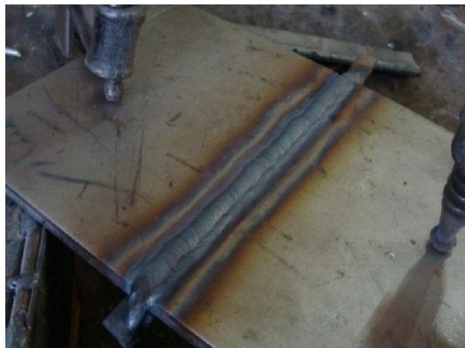
Fig. 1. a view of welded plate after welding under clamps
