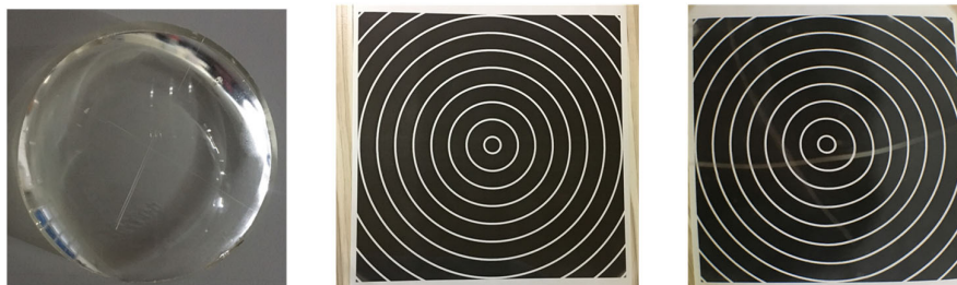
Fig. 2. A testing lens sample and two acquired imaging images using the concentric circles pattern for image acquisition
