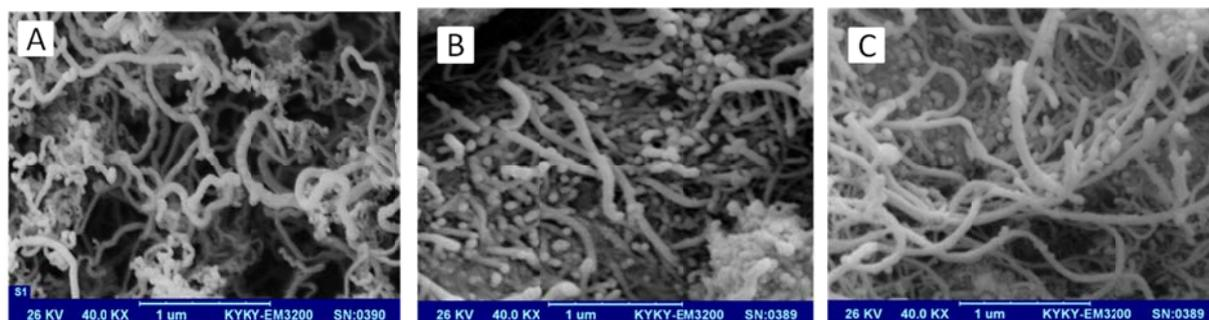
**Fig. 9.** SEM images of raw MWCNTs (A), salen2@MWCNTs (B) and salen3@MWCNTs (C)
