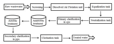
CPS: Corrugated Plate Separator , PPS: Parallel Plate Separator
